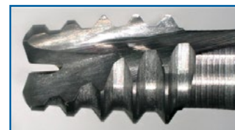
AT-2 R-SPEC after 100 Holes
