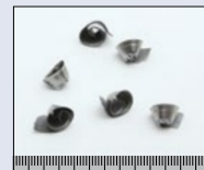
Ø20 hole processing (non-step drilling)
